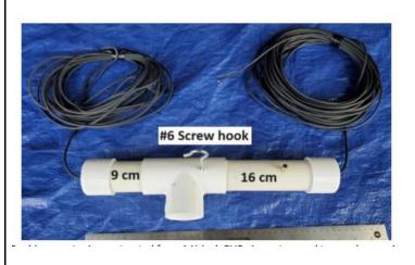
Made from pipes ppr 50, two plugs and a tee of the appropriate size. A hook is provided for gripping. A cable is attached to both sides of the repeater. The
