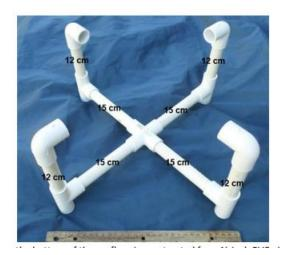
Made from pipes ppr 20 and fittings of the appropriate size. The lower part of the structure is weighted.
