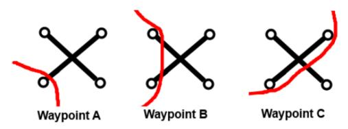
Waypoint A is an unsuccessful cable lay, as the cable is inside one vertical post only. Waypoint B is a successful cable lay, as the cable is inside two vertical posts. Waypoint C is an unsuccessful cable lay, as the cable is only inside one vertical post (the lower right post only).
