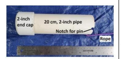
Made from a 20 cm long PPR 63 tube with a plug (can be replaced with a 50 mm tube and a corresponding plug). A rope with a loop at the end is tied to the buoy. The length of the rope is no more than half the depth of the pool (<1 m). At the end of the rope there is a loop for attaching a pin. There are also slots on both sides of the displacer for installing a pin.
