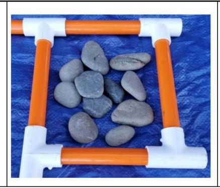
The sediment sample consists of Beach Pebbles with Velcro hooks attached.
