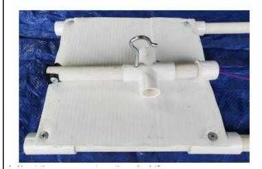
Made from a PPR 20 tube, a tee and a plug. For ease of gripping, a hook is installed in the tee. A 4 m long rope is attached to the plug (the length can be shortened. The other end of the rope is tied to the docking station. Velcro tape (hooks) is attached to the end of the connector. The connector is weighted and is initially located on the docking station platform.
